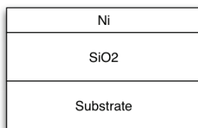
Fig. 5. Schematic diagram of the sample prepared for graphene growth. The top Ni layer is the catalyst, and the middle layer SiO 2 is the diffusion barrier layer to prevent Ni diffusion to the substrate that is usually silicon.
